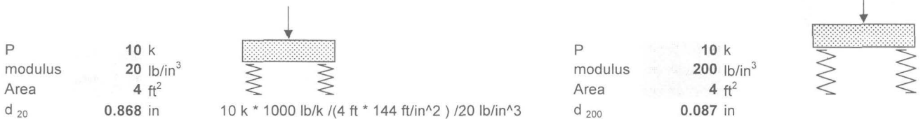
Figure 29-2 Deflections as governed by soil modulus.
