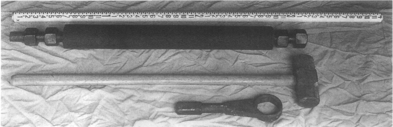
Figure 25-11 The 1 1/2" Ø bolt in an epifoam insulation sleeve is shown here with a 10 Lb. hammer and hit wrench. The surveyor's rod is used for reference.
