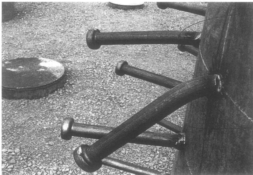
Figure 49-4 Testing the weld stud with a BFH (big fat hammer).
